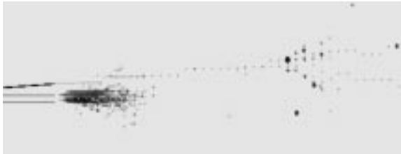
Figure 7. Simulation of a 300 GeV \tau with the decay mode \tau \rightarrow \rho\nu \rightarrow \pi^+\pi^0\nu in the TESLA Si/W ECal and digital HCal. Figure from H. Videau.
